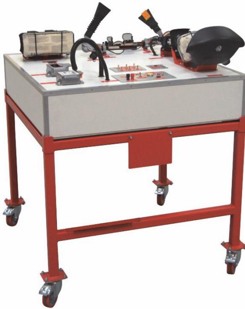
This demonstration unit utilizes real components to show the construction and operation details of air bag supplemental restraint systems. This system is ideal for informing students about the technology involved in these types of supplemental restraint systems. The steering wheel unit has been carefully sectioned to show the internal layout and construction of a typical restraint unit.
