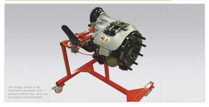
This trainer provides a fully operational disc air brake assembly for group or whole-class demonstration.
