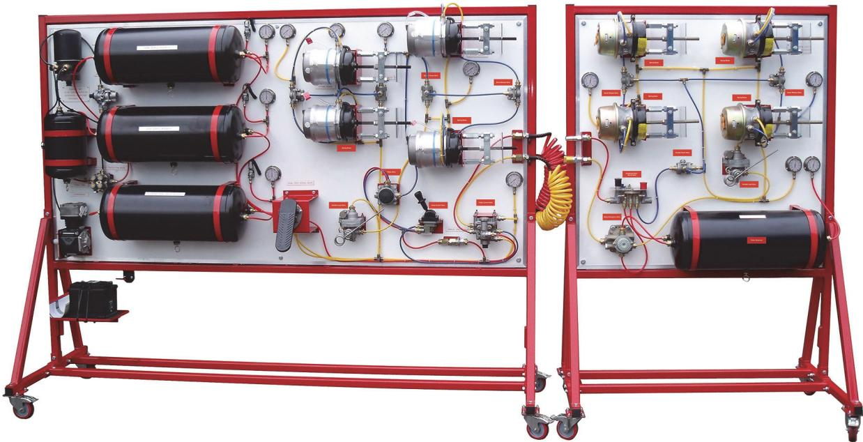
This comprehensive, panel-mounted system provides a fully operational 2-line air brake system, as fitted to a typical heavy vehicle tractor and trailer unit.
