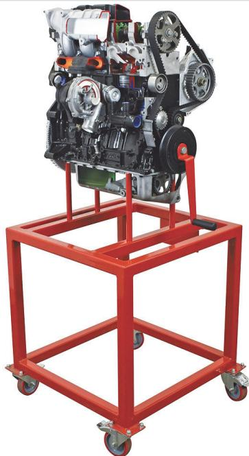
This trainer provides the instructor with a complete 4-cylinder diesel engine for group or whole-class demonstration, mounted on a moveable, heavy-duty steel frame. The engine is operated by hand and is sectioned so that all moving parts can be seen and the way they interact can be observed.
