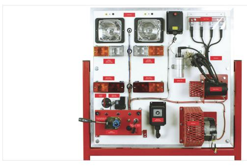
This real component trainer offers a fully operational automotive electrical system designed for teaching basic electrical principles. Investigations and demonstrations allow students to acquire an understanding of how simple electrical circuit theory is key to developing sound automotive fault-finding techniques.
