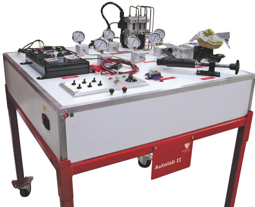
This trainer will provide the instructor with a simulated anti-lock braking system for group or whole-class demonstration, using components from a commercial ABS.
