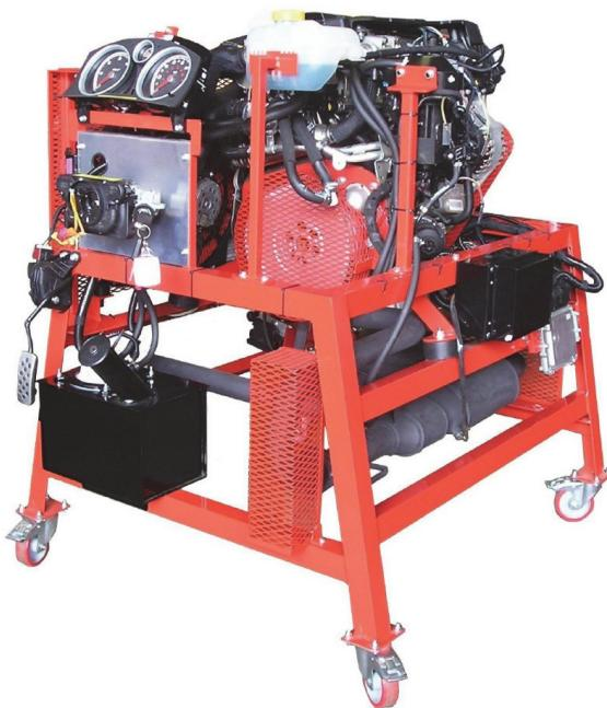
This trainer provides the instructor with a complete common rail diesel engine with an engine management system for group or whole-class demonstration. It is mounted on a moveable, heavy-duty, steel frame. The system comprises all the elements that control the injector timing and the exhaust emissions together with the ECU and all the sensors and actuators associated with the control system.
