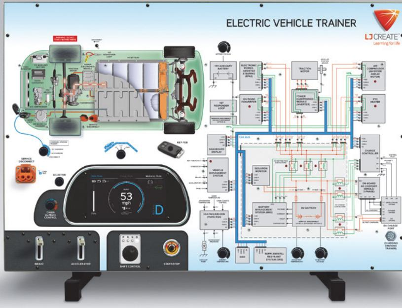
The Electric Vehicle Systems Panel Trainer provides students and instructors with the opportunity to demonstrate, investigate and fault-find a simulation of an electric vehicle electrical system.
