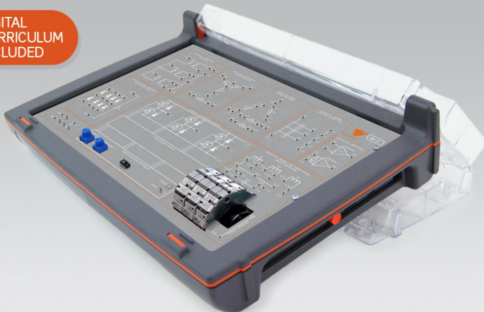
The 3-Phase Control Systems Trainer is a rugged, self-contained hardware unit that enables students to investigate practically and safely the generation of a 3 Phase supply and operation of a Motor and Inverter. The self-contained unit also incorporates three supply transformers.
