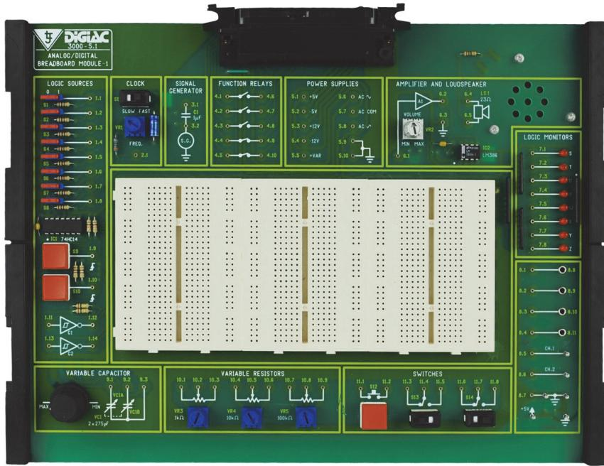
The breadboard module allows students to build a wide variety of electronic circuits using discrete components.
