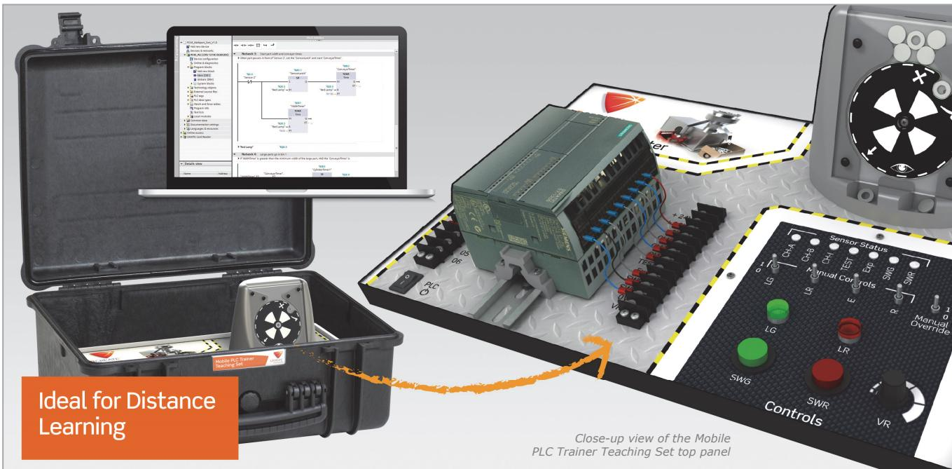
This Mobile PLC Trainer Teaching Set offers a platform that enables students to perform a comprehensive range of programming tasks culminating in the control of the unit using an industrial programmable logic controller (PLC).
