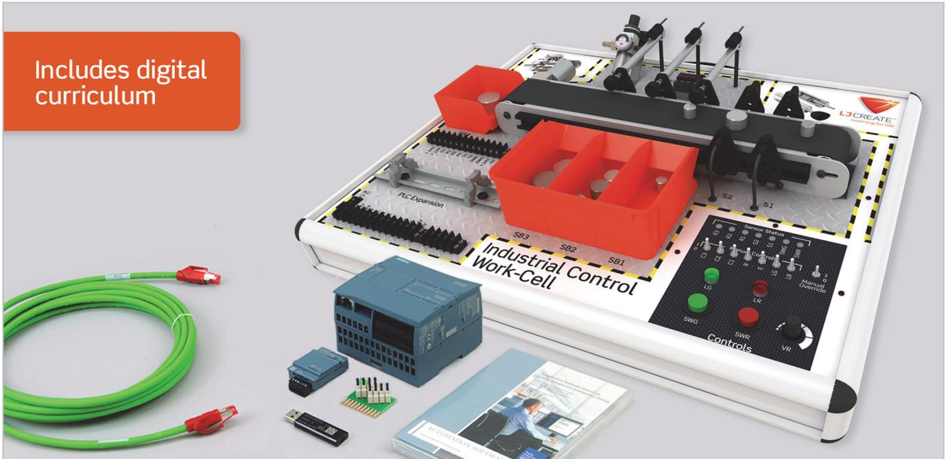
This training system offers a platform that enables students to perform a comprehensive range of PLC programming tasks using a Siemens controller and a conveyor belt/pneumatic sorting application.
