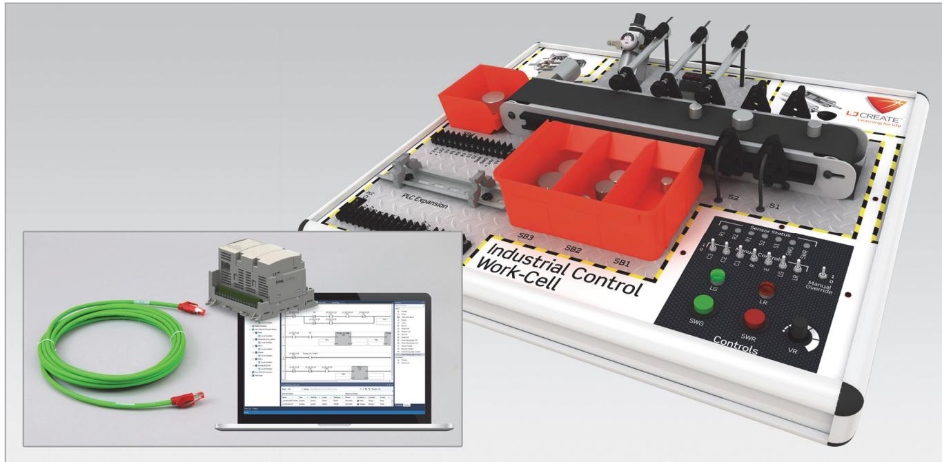
This training system offers a platform that enables students to perform a comprehensive range of PLC programming tasks using an Allen Bradley controller and a conveyor belt/pneumatic sorting application.
